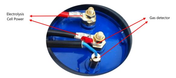
Fig 5 – Electrolysis Cell Connection Terminals
