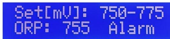
**Figure 6 - Main Menu with an Active Alarm**
